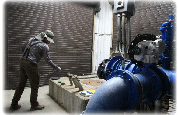
WM Staff Taking a Groundwater Level Measurement
