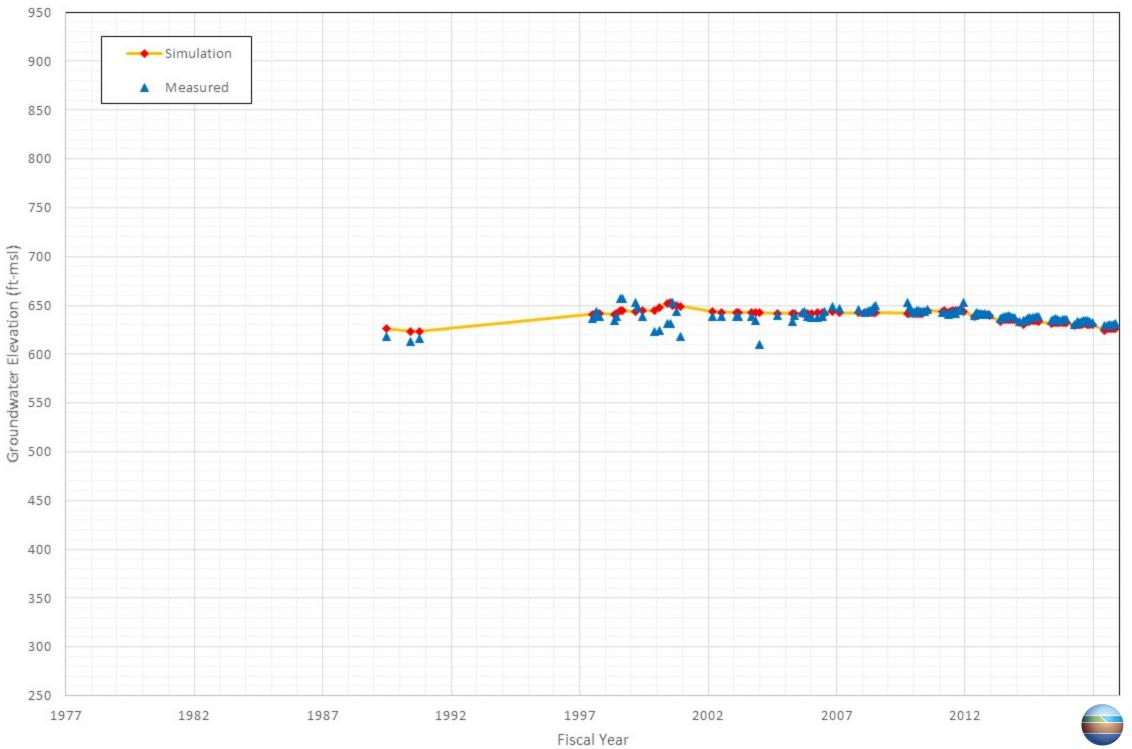
Appendix C-102 Comparison of Measured and Simulated Groundwater Water Level in the California State Polytechnic University, Pomona's Well Well 1
