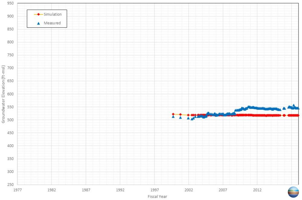
Appendix C-96 Comparison of Measured and Simulated Groundwater Water Level in the Unknown's Well AG#6-BRITSCHGI
