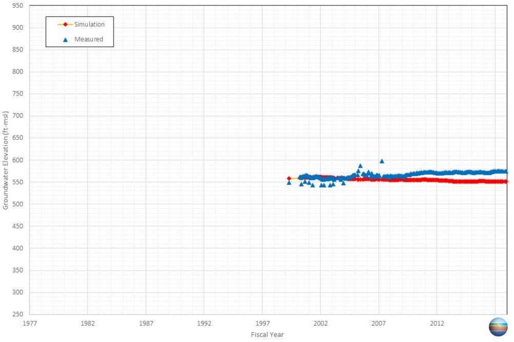
Appendix C-93 Comparison of Measured and Simulated Groundwater Water Level in the Stark, Everett's Well 74200-IRR
