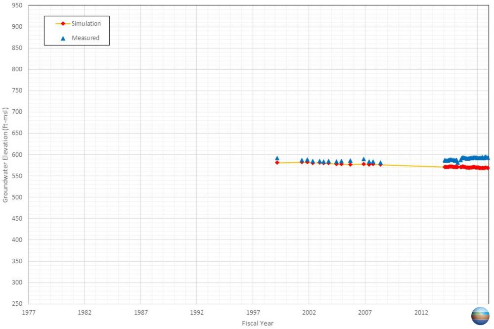
Appendix C-87 Comparison of Measured and Simulated Groundwater Water Level in the H & R Barthelemy Dairy's Well ABANDONED
