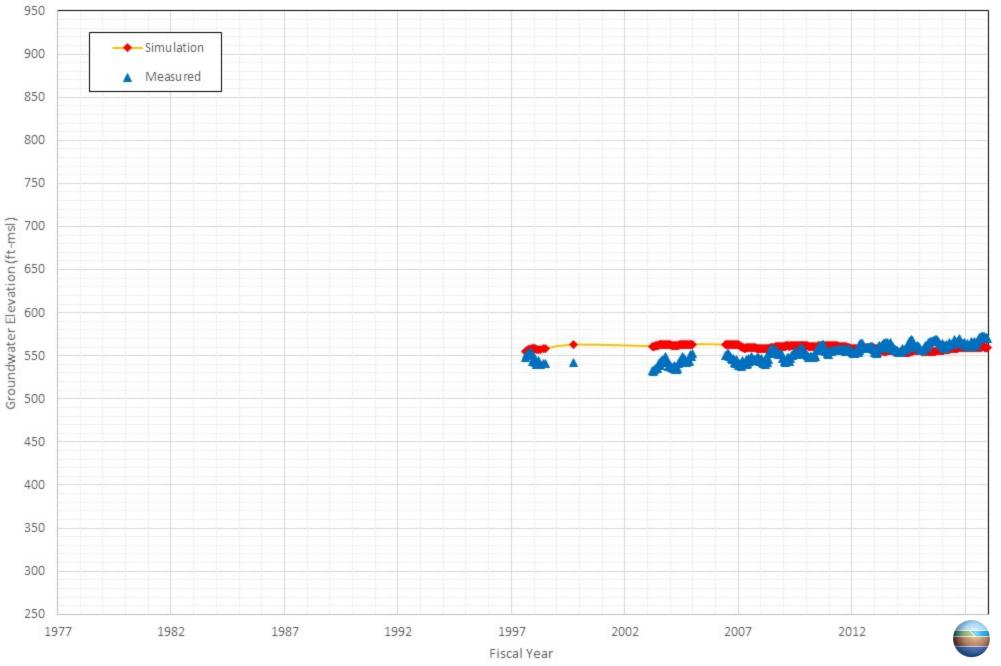
Appendix C-74 Comparison of Measured and Simulated Groundwater Water Level in the State of California, Department of Toxic Substances Control's Well FC-936A2
