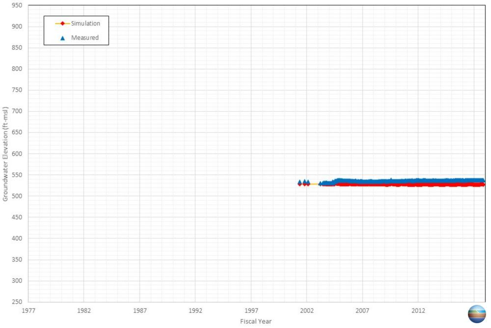
Appendix C-76 Comparison of Measured and Simulated Groundwater Water Level in the West End Consolidated Water Co.'s Well West End 1
