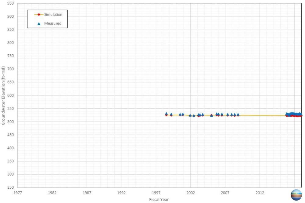
Appendix C-84 Comparison of Measured and Simulated Groundwater Water Level in the En Sue, Liau's Well DOM
