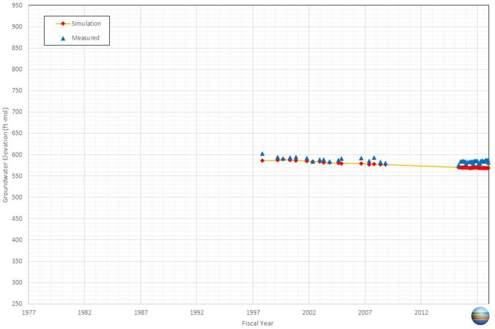
Appendix C-80 Comparison of Measured and Simulated Groundwater Water Level in the Borba, John's Well 9200-DOM
