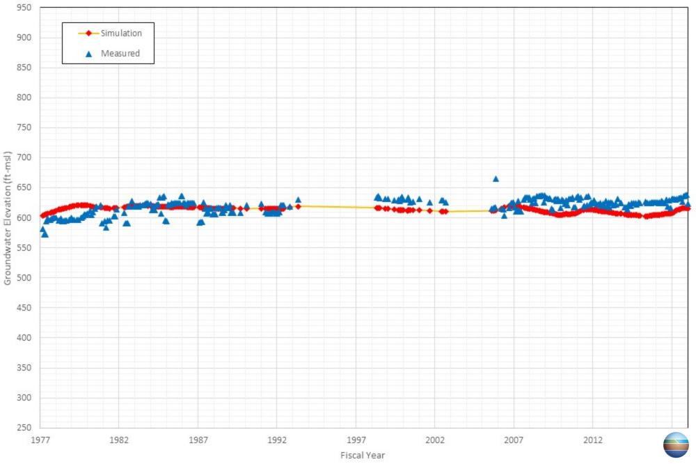
Appendix C-70 Comparison of Measured and Simulated Groundwater Water Level in the State of California, California Institution for Men's Well 03
