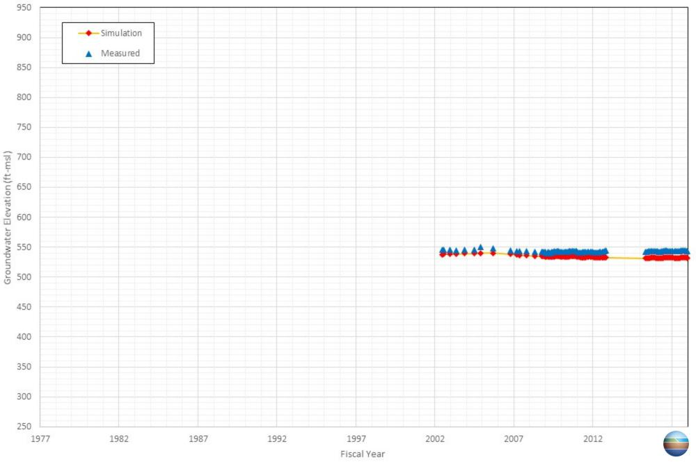
Appendix C-95 Comparison of Measured and Simulated Groundwater Water Level in the Stueve Brothers Farms's Well Dom
