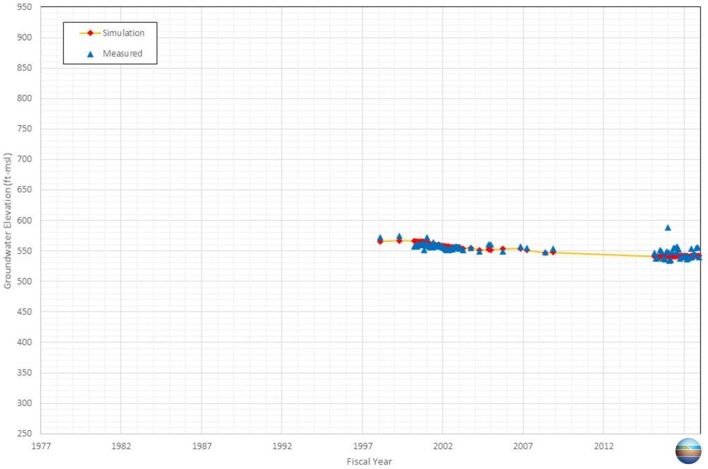
Appendix C-89 Comparison of Measured and Simulated Groundwater Water Level in the Lizzaraga, Frank's Well IRRIGATION-capped
