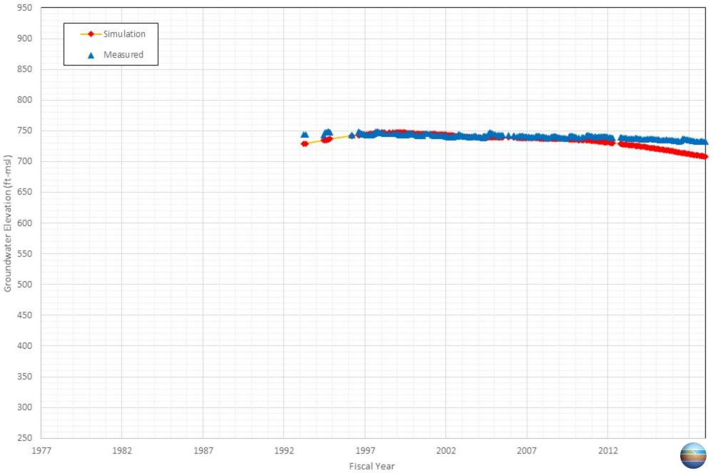
Appendix C-75 Comparison of Measured and Simulated Groundwater Water Level in the United States, Geological Survey (USGS)'s Well Archibald 1
