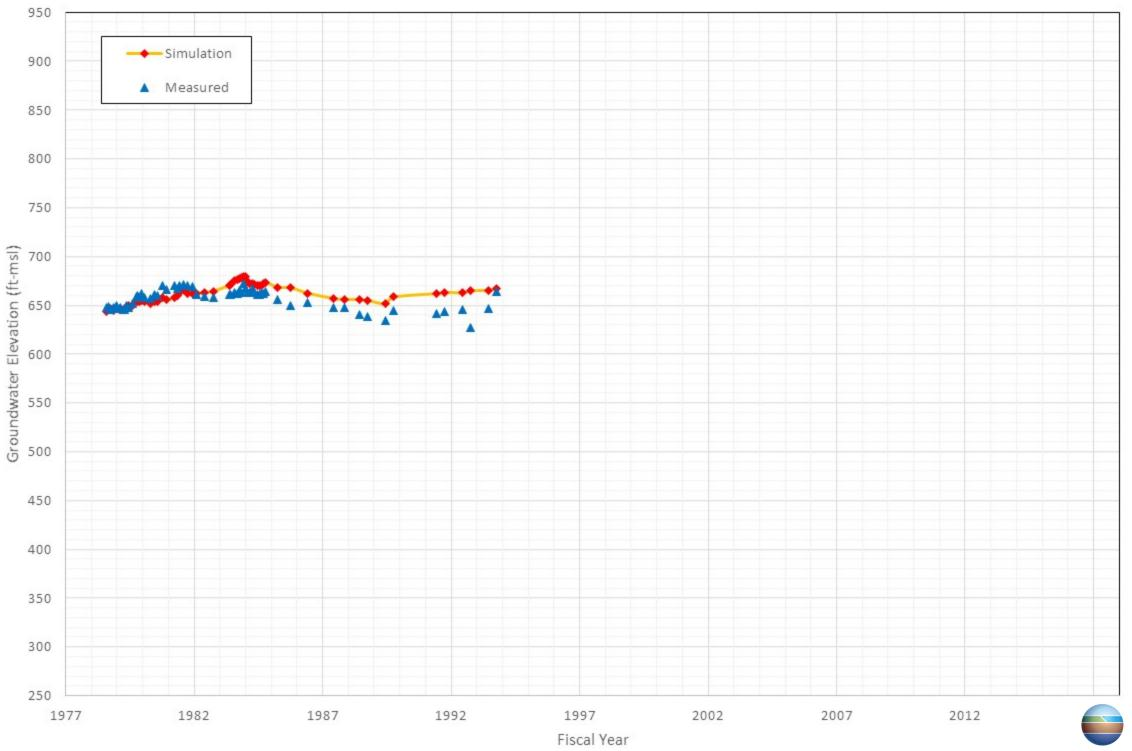
Appendix C-104 Comparison of Measured and Simulated Groundwater Water Level in the City of Pomona's Well P-31 (OGT-3)
