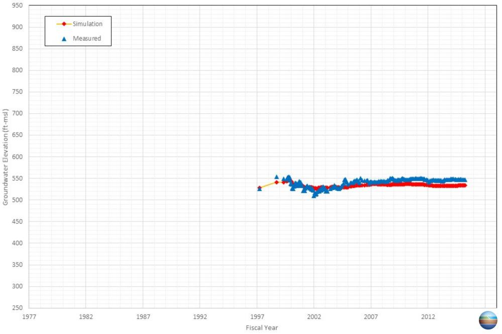
Appendix C-94 Comparison of Measured and Simulated Groundwater Water Level in the Sterling Leasing Inc's Well DOM/Office
