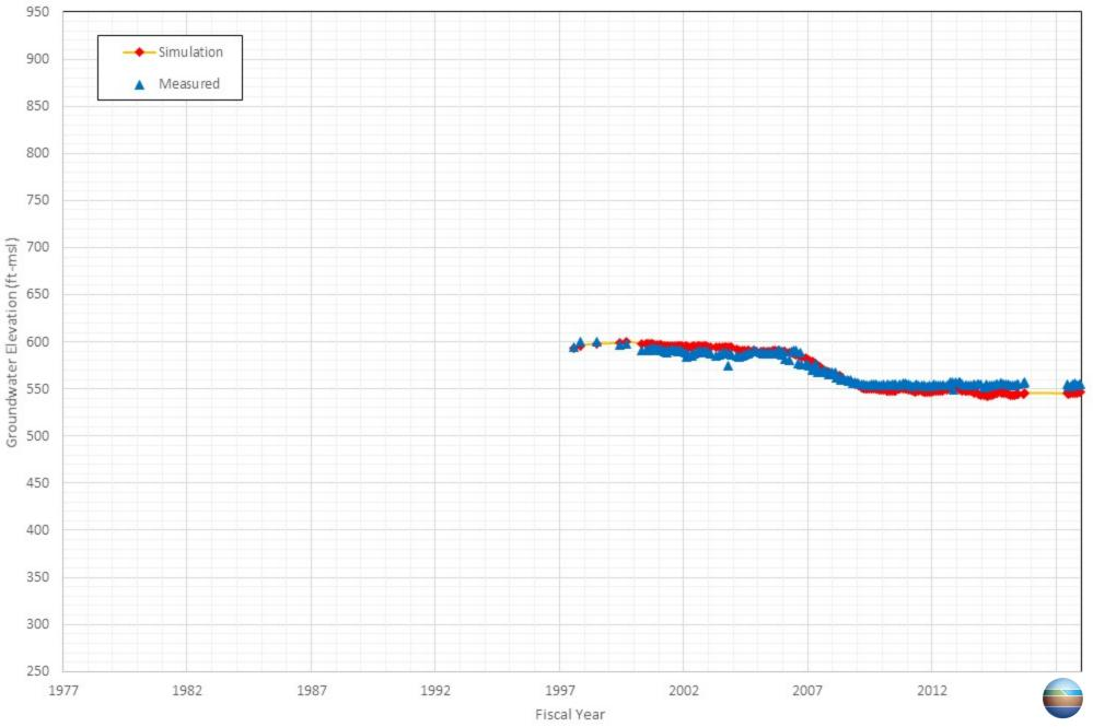
Appendix C-101 Comparison of Measured and Simulated Groundwater Water Level in the City of Pomona's Well P-28
