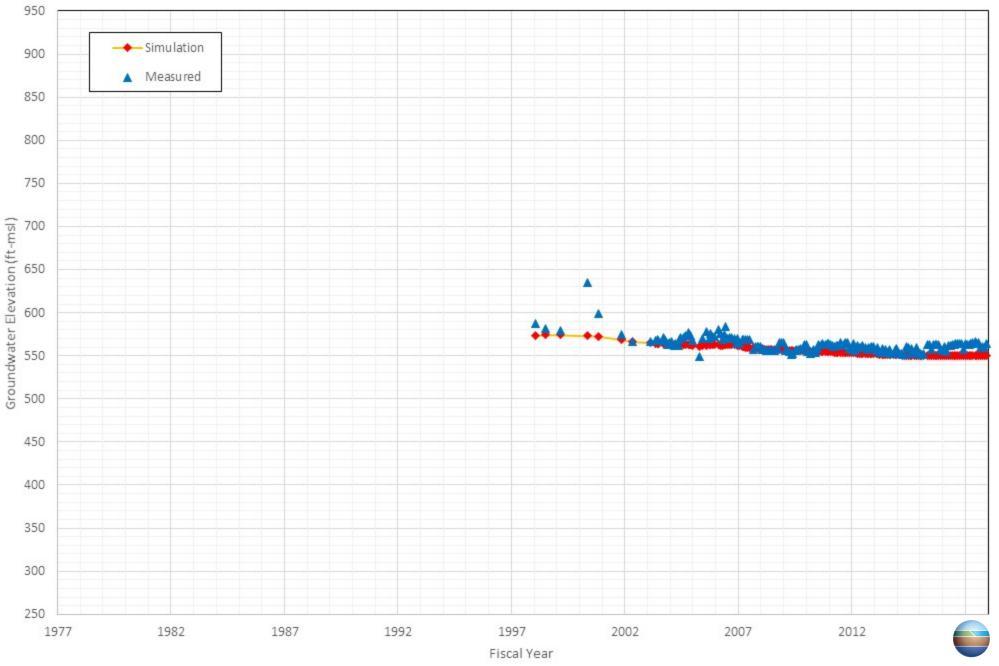
Appendix C-81 Comparison of Measured and Simulated Groundwater Water Level in the Boschma & Son Dairy's Well DOM
