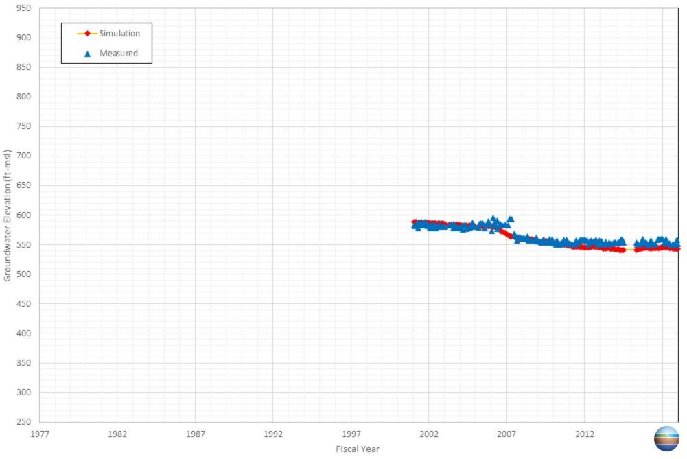
Appendix C-86 Comparison of Measured and Simulated Groundwater Water Level in the Gutierrez, Ernesto's Well NA\_1206525
