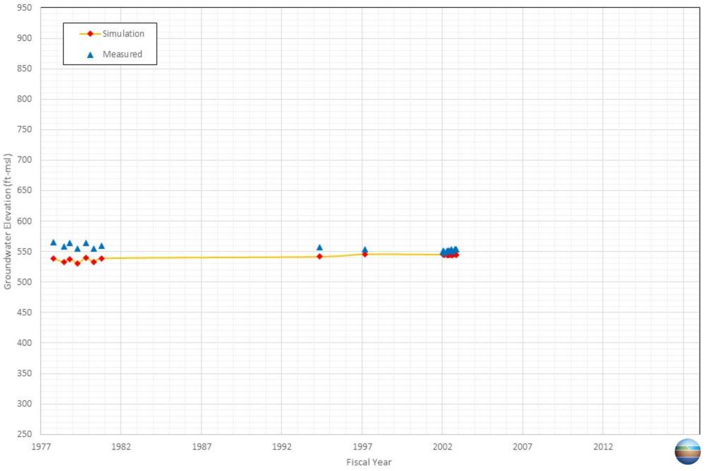
Appendix C-91 Comparison of Measured and Simulated Groundwater Water Level in the Mobile Community Management Company's Well 4
