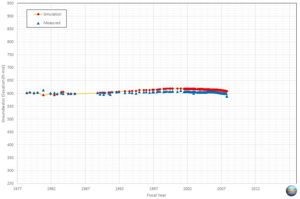
Appendix C-69 Comparison of Measured and Simulated Groundwater Water Level in the San Antonio Water Company's Well SAWC 18
