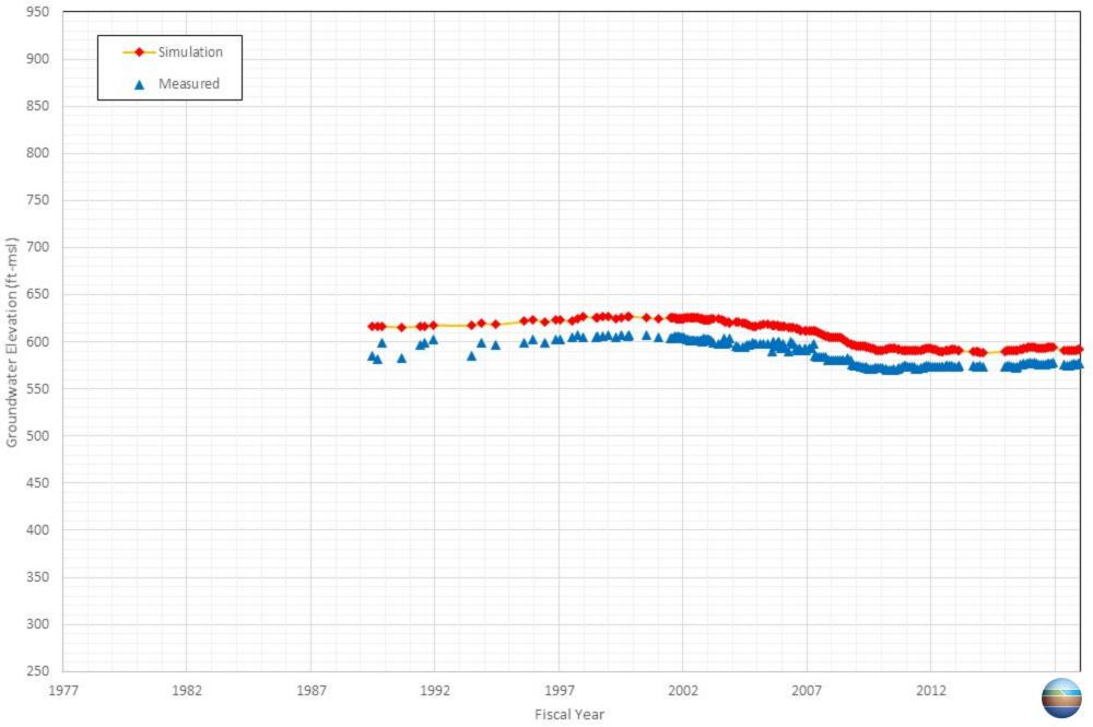
Appendix C-68 Comparison of Measured and Simulated Groundwater Water Level in the Santa Ana River Water Company's Well 07
