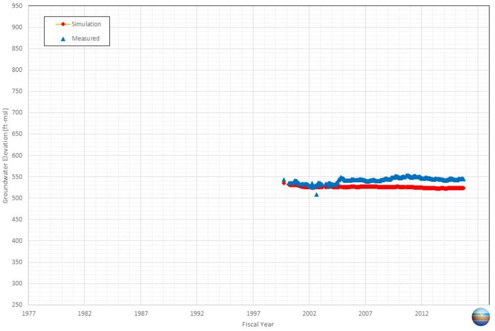
Appendix C-88 Comparison of Measured and Simulated Groundwater Water Level in the Lee, Henrietta's Well DOM
