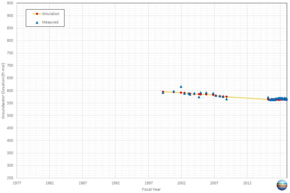
Appendix C-82 Comparison of Measured and Simulated Groundwater Water Level in the Bouma, Ewoude's Well NA\_1206751
