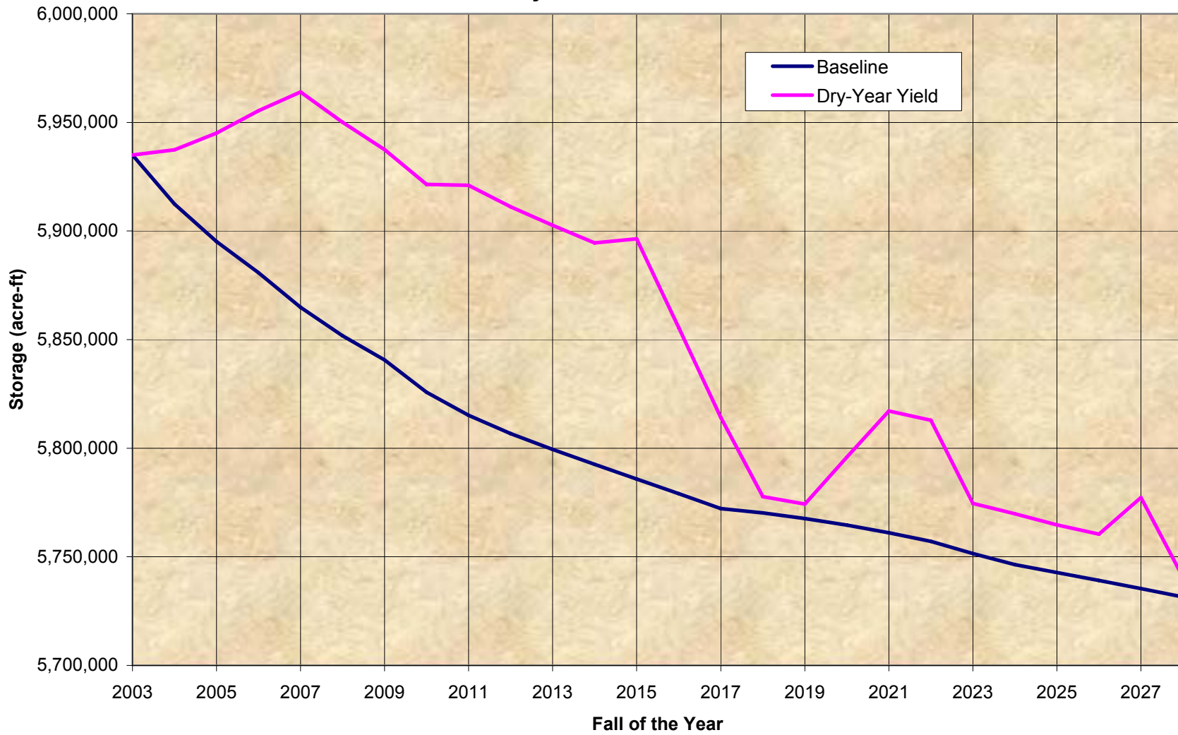
Figure 9-6 Projected Time History of Total Storage in the Chino Basin for Baseline and Dry-Year Yield Scenarios
