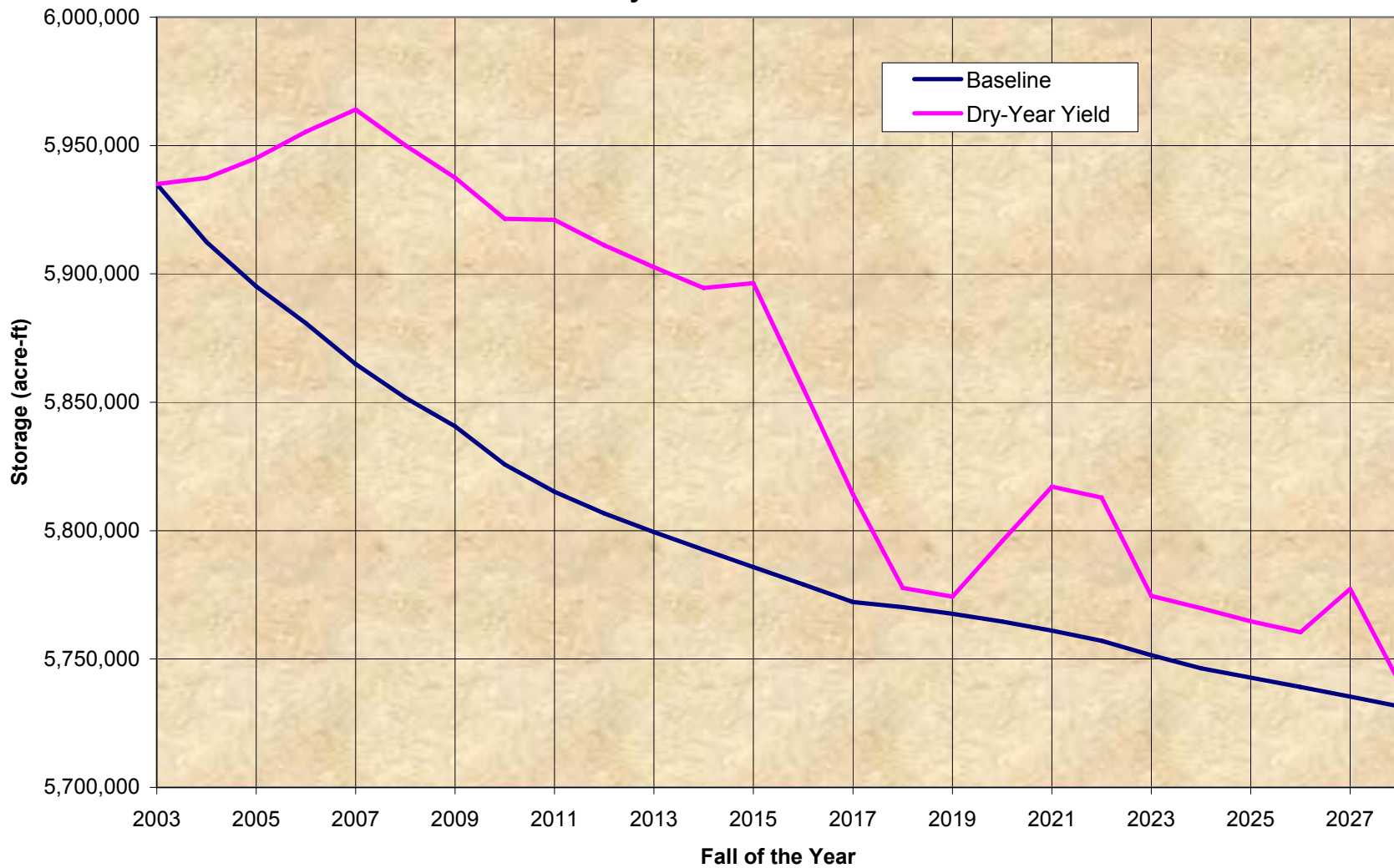
Figure 8-11 Projected Time History of Total Storage in the Chino Basin for Baseline and Dry-Year Yield Scenarios
