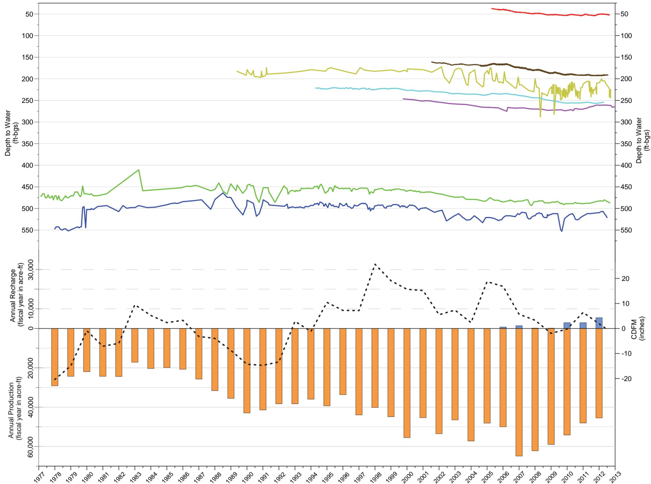
This exhibit is a time-series chart that displays groundwater levels at wells, annual production, and annual artificial recharge to basins, in MZ3, for the time period since the Judgment to FY 2011/2012. Climate is displayed as CDFM precipitation plot using the PRISM data from 1895 to 2012. Upward sloping lines on the CDFM curve indicate wet years or wet periods. Downward sloping lines indicate dry years or dry periods.
