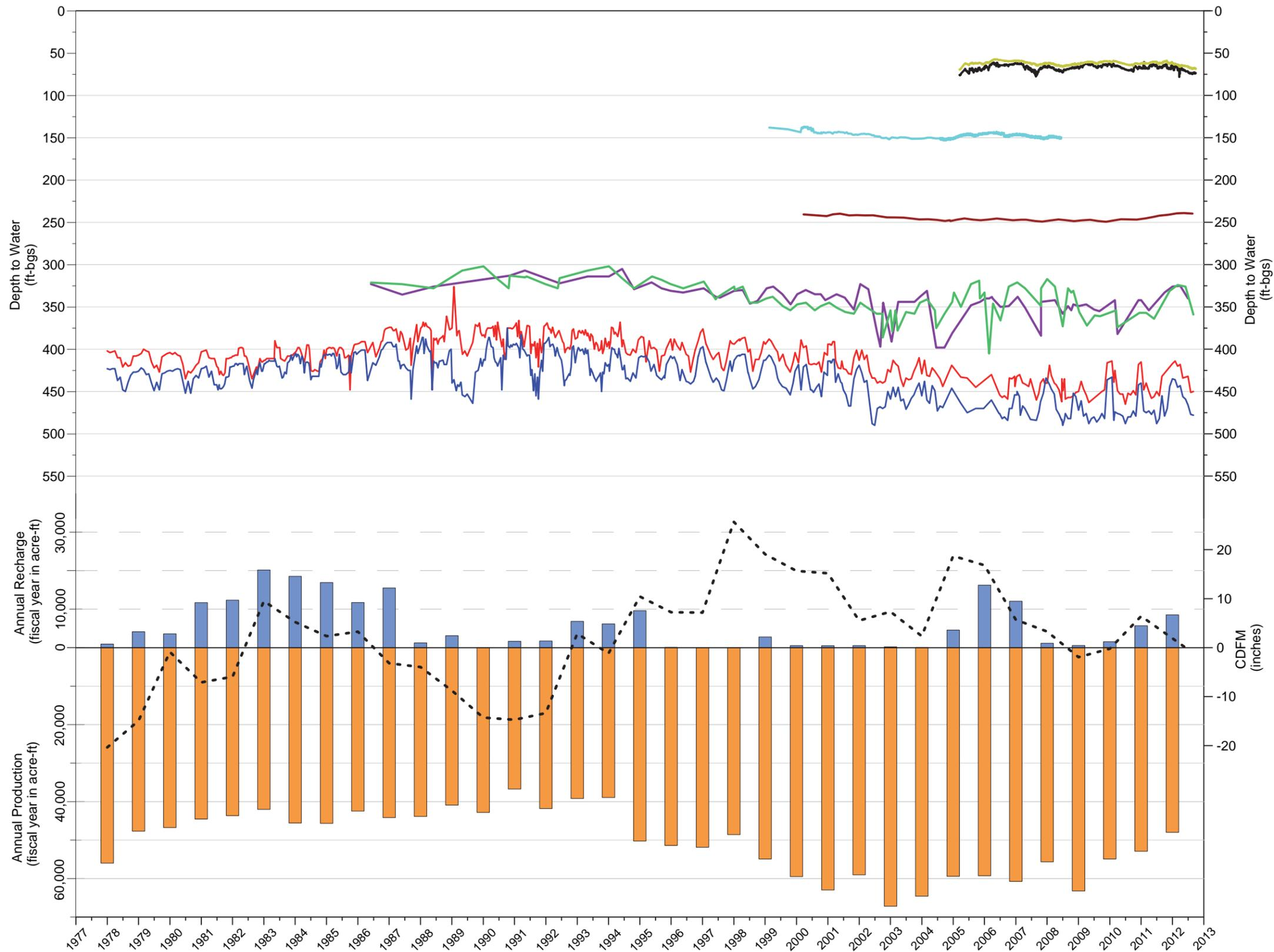
This exhibit is a time-series chart that displays groundwater levels at wells, annual production, and annual artificial recharge to basins, in MZ2, for the time period since the Judgment to FY 2011/2012. Climate is displayed as CDFM precipitation plot using the PRISM data from 1895 to 2012. Upward sloping lines on the CDFM curve indicate wet years or wet periods. Downward sloping lines indicate dry years or dry periods.
