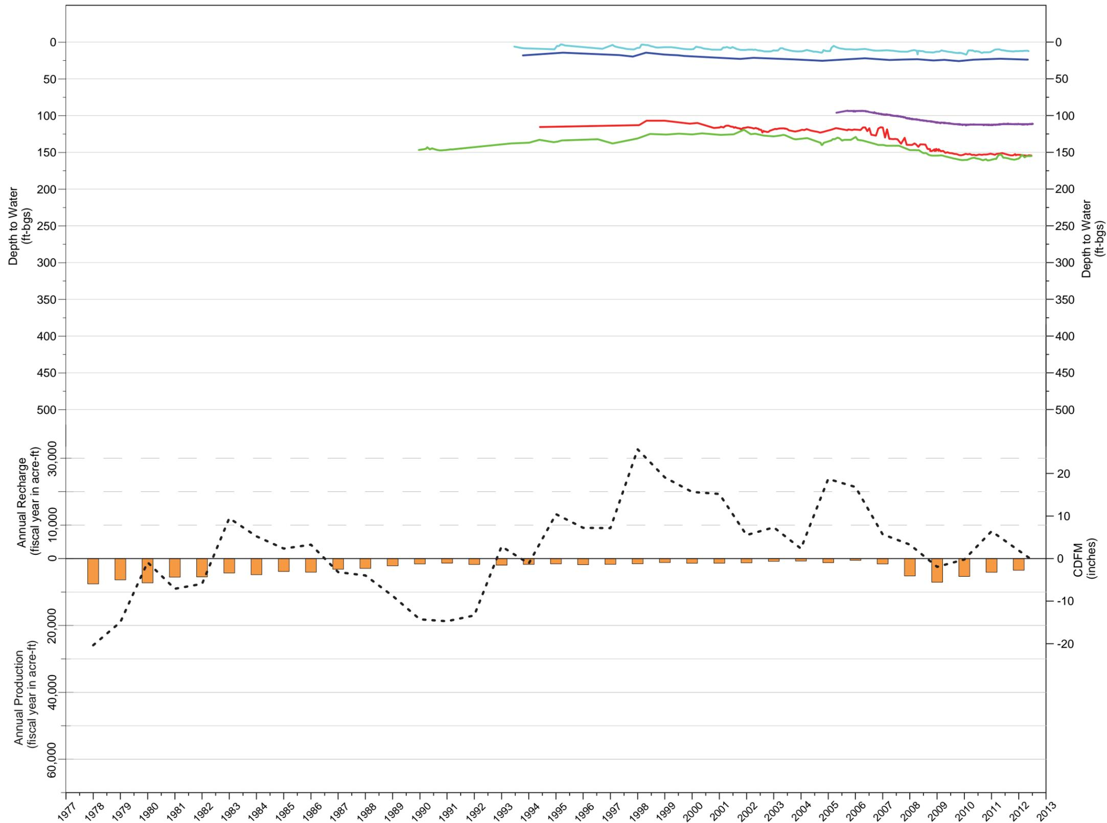
This exhibit is a time-series chart that displays groundwater levels at wells, annual production, and annual artificial recharge to basins, in MZ4, for the time period since the Judgment to FY 2011/2012. Climate is displayed as CDFM precipitation plot using the PRISM data from 1895 to 2012. Upward sloping lines on the CDFM curve indicate wet years or wet periods, and downward sloping lines indicate dry years or dry periods.
