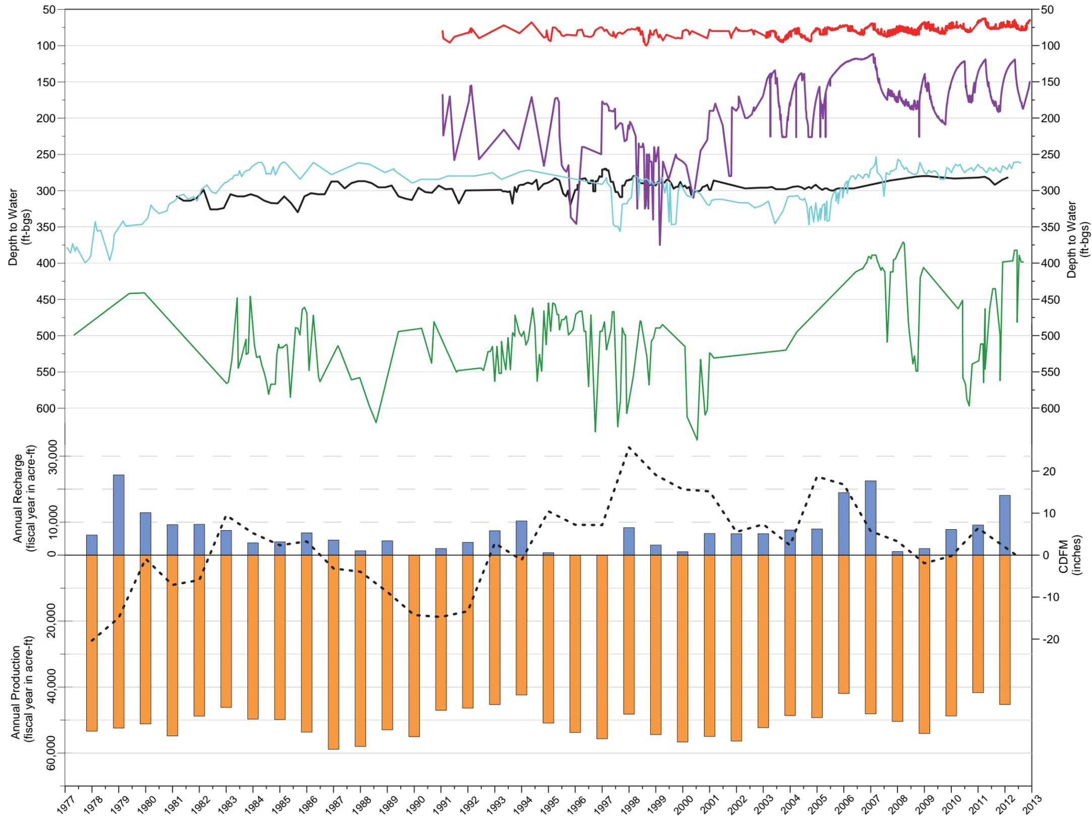
This exhibit is a time-series chart that displays groundwater levels at wells, annual production, and annual artificial recharge to basins, in MZ1, for the time period since the Judgment to FY 2011/2012. Climate is displayed as CDFM precipitation plot using the PRISM data from 1895 to 2012. Upward sloping lines on the CDFM curve indicate wet years or wet periods. Downward sloping lines indicate dry years or dry periods.
