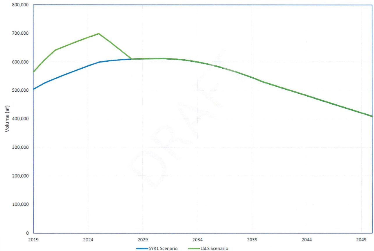
Figure 2-2. Planned End-of-Year Volume in Managed Storage for the SYR1 and LSLS Scenarios
