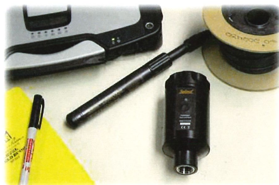
Pressure Transducer Equipment Before Installation
